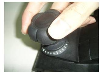
**CAUTION:** Always ensure that the number on the ring is at the "0" position when the tool is not in use; at this position, the blade can not cut the workpiece.
