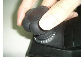
Rotate the depth adjustment knob clockwise for a deeper cut and counter-clockwise for a shallower cut.
